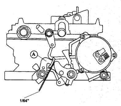
With the primary and secondary throttle valves tightly closed, there should be 1/64" clearance between the levers as shown. To adjust, bend the shoe on the lever (A).
