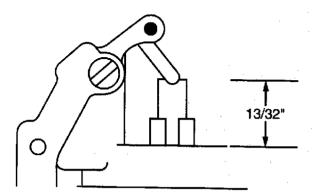
Back out the throttle speed screw (count turns) to allow throttle valves to seat in the bores. Install connector rod in the second from the bottom hole of the pump lever. Adjust rod to obtain 13/32" from top of the bowl cover to the top of the plunger stem as shown.
