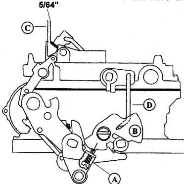
Place fast idle screw (A) on second step of cam (B). Move choke valve towards the closed position as far as possible without forcing. The dimension (C) should be 5/64" between the upper edge of the choke valve and the wall of the air horn. To adjust bend rod (D).
