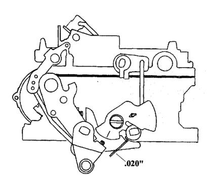
Crack the throttle valves and manually open and close the choke valve. The tang on the secondary throttle lever should freely engage in the notch of the lock out dog. To adjust, bend the tang on the secondary throttle lever.
