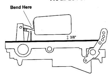
With the bowl cover inverted, bowl cover gasket in place, and weight of float seating on the needle, there should be 3/8" between the top of each float and the bowl cover gasket (at the outer end on the seam). The sides of the floats should be parallel to the outer edge of the bowl cover. To adjust, bend the float lever near the pivot pin.
