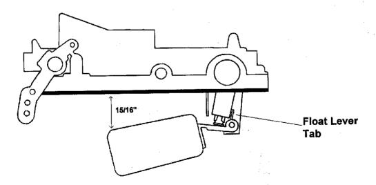
With the bowl cover held in the upright position adjust stop tabs on the float brackets to obtain 15/16" between the outer end of each float and bowl cover gasket. To adjust, bend the tab on the float lever.
