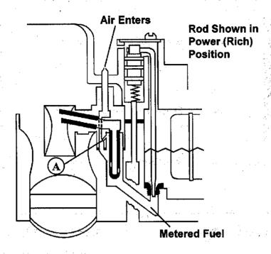
Fuel for part throttle and full throttle operation is supplied by the high speed circuit.
