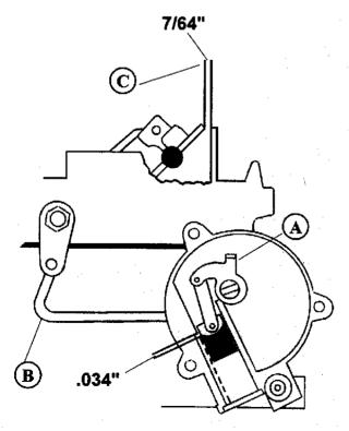
Open the choke valve and insert a .034" wire (paper clip) (bend 90 degrees 1/8" from the end) between top of slot in the choke piston cylinder and the bottom of the slot in the piston. Hold the wire in position and close choke valve by pressing on the piston (A) until resistance is felt. The dimension (C) should be 7/64" between the top edge of the choke valve and the wall of the air horn. To adjust bend rod (B). Reassemble the thermostatic choke coil to the housing.
