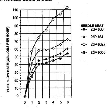
FUEL PRESSURE (PSI) HIGH RPM CONDITIONS
