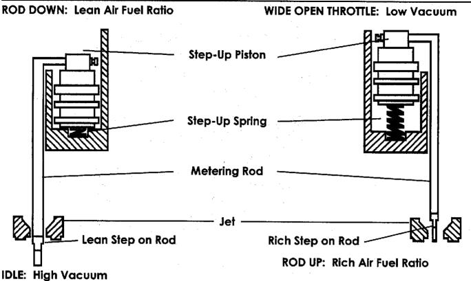
The use of wrong step-up piston spring, or one that has been stretched or cut off, can seriously upset carburetor calibration.
