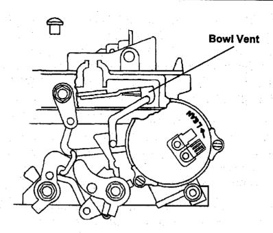
The AFB series emission calibrated carburetors use a combination of a mechanically operated internal and external vents. The non-emission calibrated and marine carburetors use an internal vent only.
