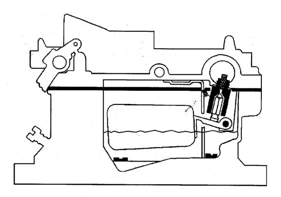
The purpose of the float circuit is to maintain an adequate supply of fuel at the proper level for use by the low speed, high speed, accelerator pump and choke circuits.
